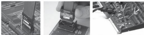
Figure 2.61 Logic-analyzer probes. © Tektronix.
