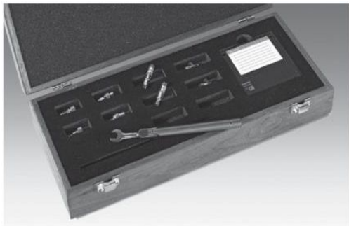
Figure 2.50 A calibration box. © Agilent.
