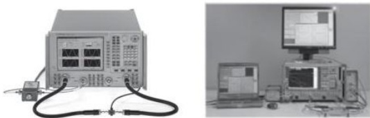
Figure 2.52 Two mixer-based NVNAs. Images © external vendors.
