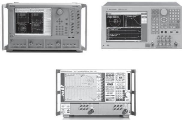
Figure 2.46 Two-port VNAs: from left to right, Anritsu, Agilent Technologies, and Rohde & Schwarz. © Anritsu, Agilent Technologies, and Rohde & Schwarz.
