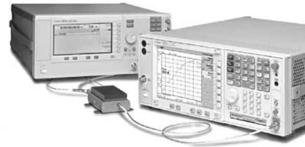
Figure 12.2 Photograph of a high-performance spectrum analyser based scalar network analyzer, which uses a high-performance external source as the tracking generator
