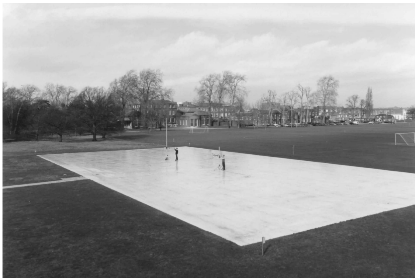
Figure 19.1 The 60 × 30 m ground plane at the National Physical Laboratory, Teddington, UK, whose surface is flat to within \pm 15 mm over 95 per cent of its area
